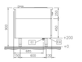
D = Drain EI = Electrical inlet (power) EQ = Equipotential screw WI = Water inlet
